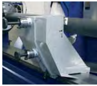
Steady rest capacity \varnothing 30 -180 mm
