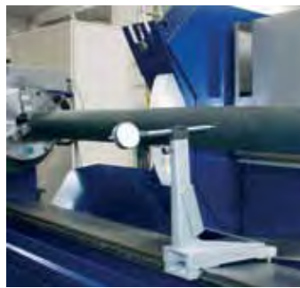
Set-up indicator with quick set dial gauge
