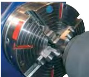
Self-centering chucks with adjustable jaws
