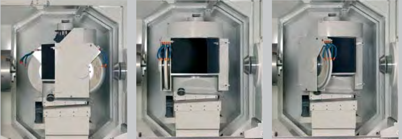
Swivelable CNC B-axis for automatic positioning of the wheelhead at any desired angle.
